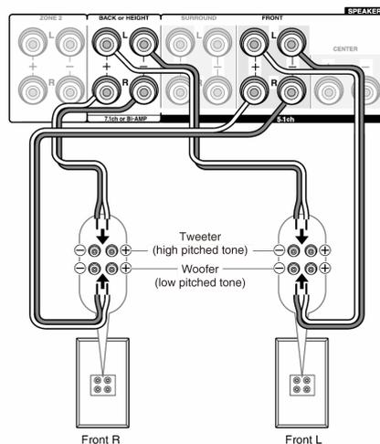
2. Turn the unit on and set "Speaker Setup" to "Bi-Amp".
