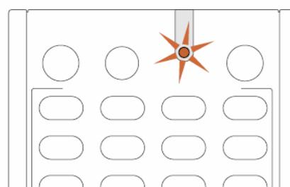
3. With the number buttons, enter the 5-digit remote control code within 30 seconds.
