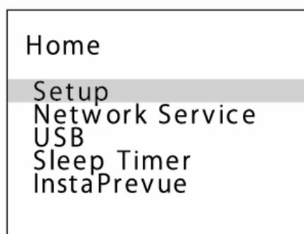
2. Select "Setup" - "10. Hardware" - "Update via NET" in order using the cursor buttons, and then press ENTER.
