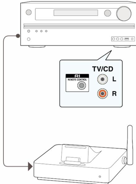
Connect an Onkyo component with RI jack to the unit using an RI cable and an analog audio (RCA) cable. For details, refer to the instruction manual of the component with RI jack. The RI cable can be connected in any order. When there are two RI jacks, you can connect to either one as both jacks work in the same way.
