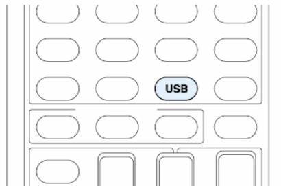
2. Plug your USB storage device with the music files into the USB port of the unit, so that the "USB" lights on the display.
