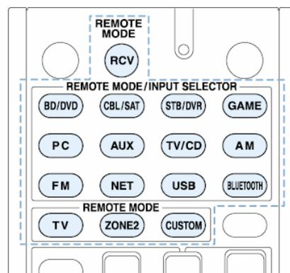
\* The RCV and ZONE2 buttons cannot be programmed.
