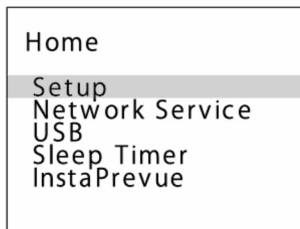
7. Select "Setup" - "10. Hardware" - "Update via USB" in order using the cursor buttons, and then press ENTER.
