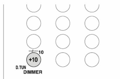
3. Using the number buttons, enter the frequency of the radio station within 8 seconds.
