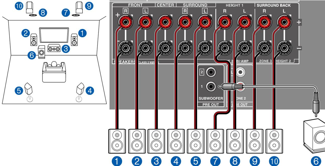
This is an example of combining the top middle speakers at the front and the rear high speakers at the rear to the 5.1 Channel System. The height speakers in front can be selected from following 4 types. The height speakers that can be combined at the rear differ depending on the height speakers used at the front.
