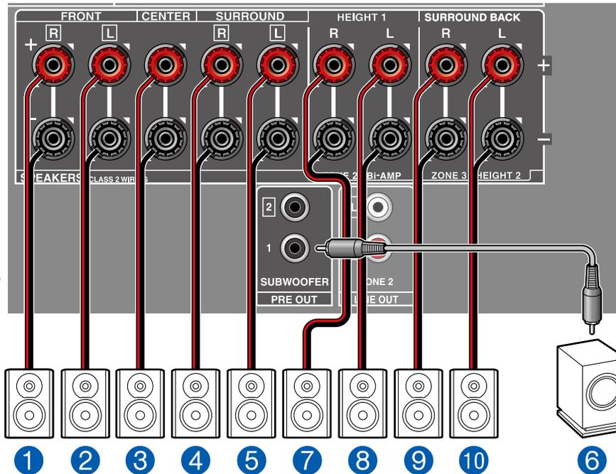
**MAIN ROOM:** This is a basic 5.1 Channel System. For details of the speaker layout, refer to "Speaker Installation" (→p14).
