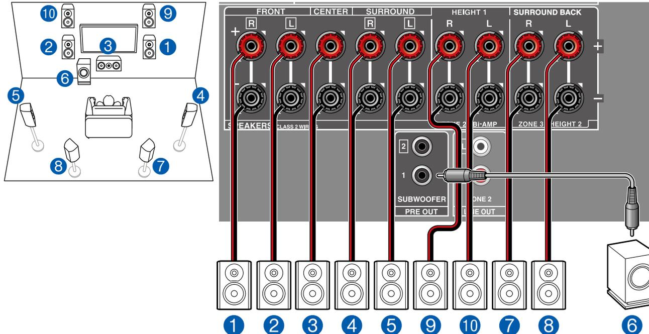
This is a combination of the 7.1 Channel System and front high speakers. A front high speaker is a type of height speaker. You can select only one set of height speakers from the following three types for connection.
