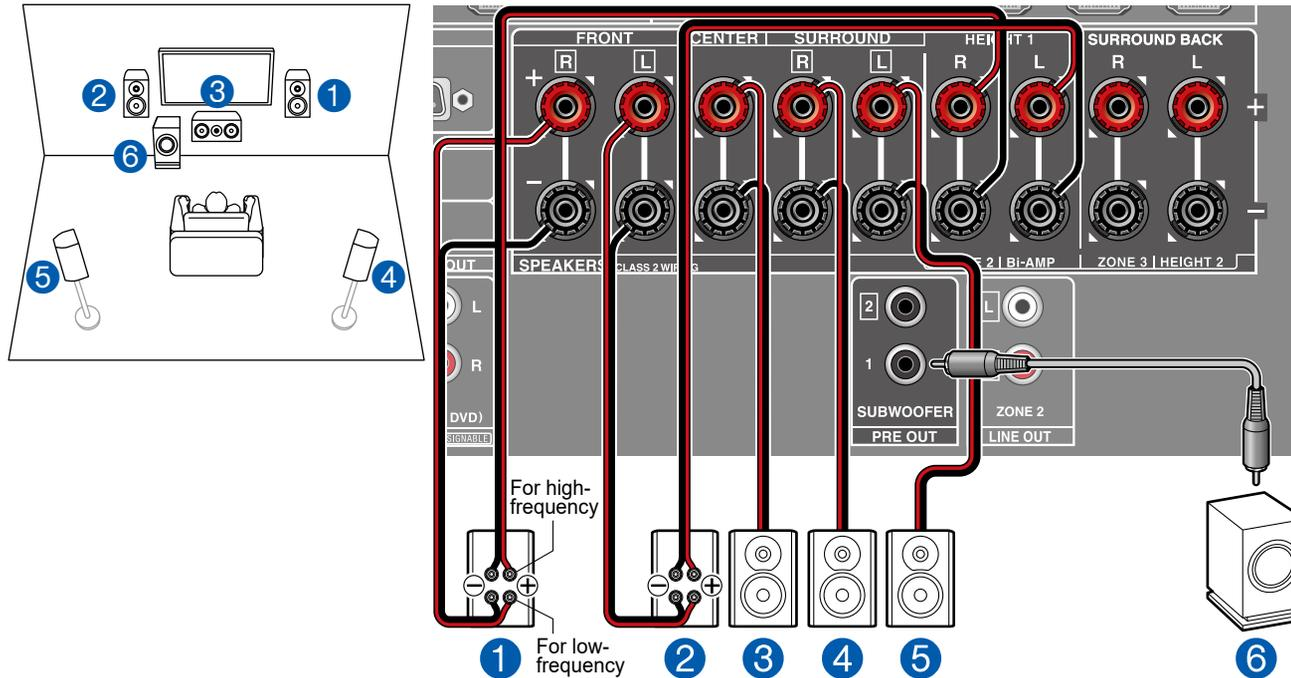
You can configure a 5.1 Channel System (→p14) by connecting front speakers that support Bi-Amping connection. The Bi-Amping connection can improve the quality of the low and high pitched ranges. Be sure to remove the jumper bar connecting between the woofer jacks and tweeter jacks of the Bi-Amping supported speakers. Refer to the instruction manual of your speakers as well.
