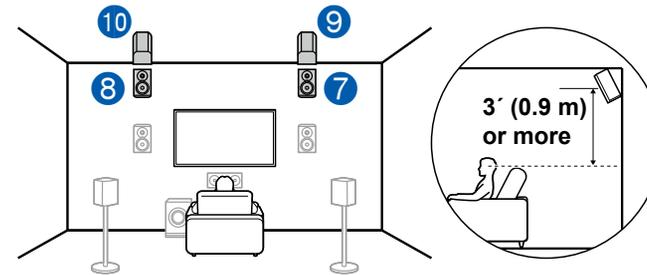
The width between the rear high speakers should match the one for the front speakers, and they should be installed minimum of 3'/0.9 m higher than the front speakers, and tilted so they will point toward the listener.
