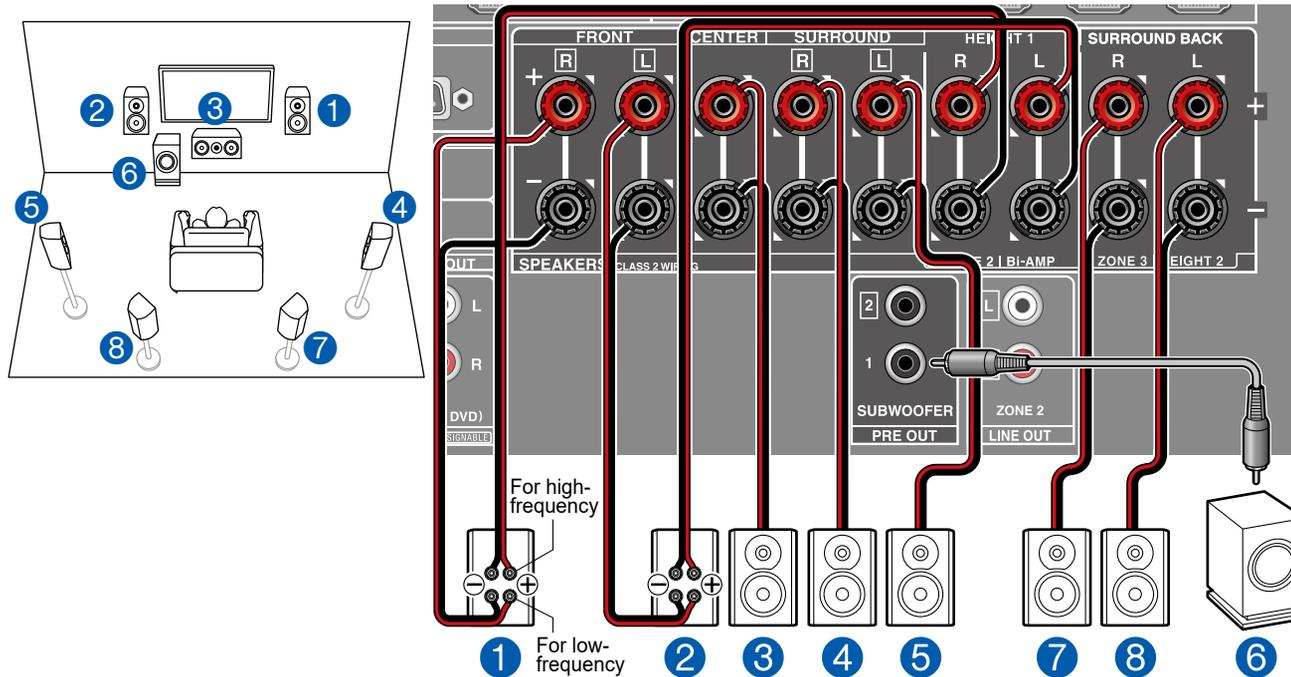
You can configure a 7.1 Channel System (→p15) by connecting front speakers that support Bi-Amping connection. The Bi-Amping connection can improve the quality of the low and high pitched ranges. Be sure to remove the jumper bar connecting between the woofer jacks and tweeter jacks of the Bi-Amping supported speakers. Refer to the instruction manual of your speakers as well.
