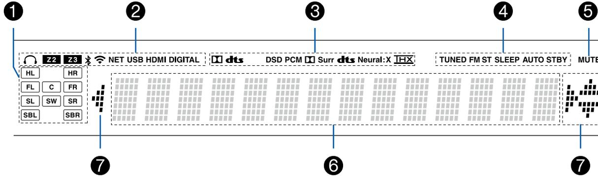
1. Speaker/Channel display: Displays the output channel that corresponds to the selected listening mode.
