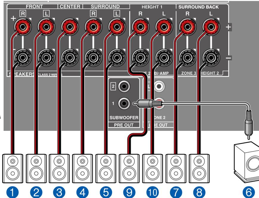
**MAIN ROOM:** This is a combination of the 5.1 Channel System and front high speakers. A front high speaker is a type of height speaker. You can select only one set of height speakers from the following three types for connection.
