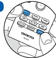
**If the remote controller does not work:** The remote controller may have switched to the ZONE control mode. While pressing and holding MODE, press the MAIN button for 3 seconds or more until the remote indicator blinks once, and then switch it to the main room control mode.
