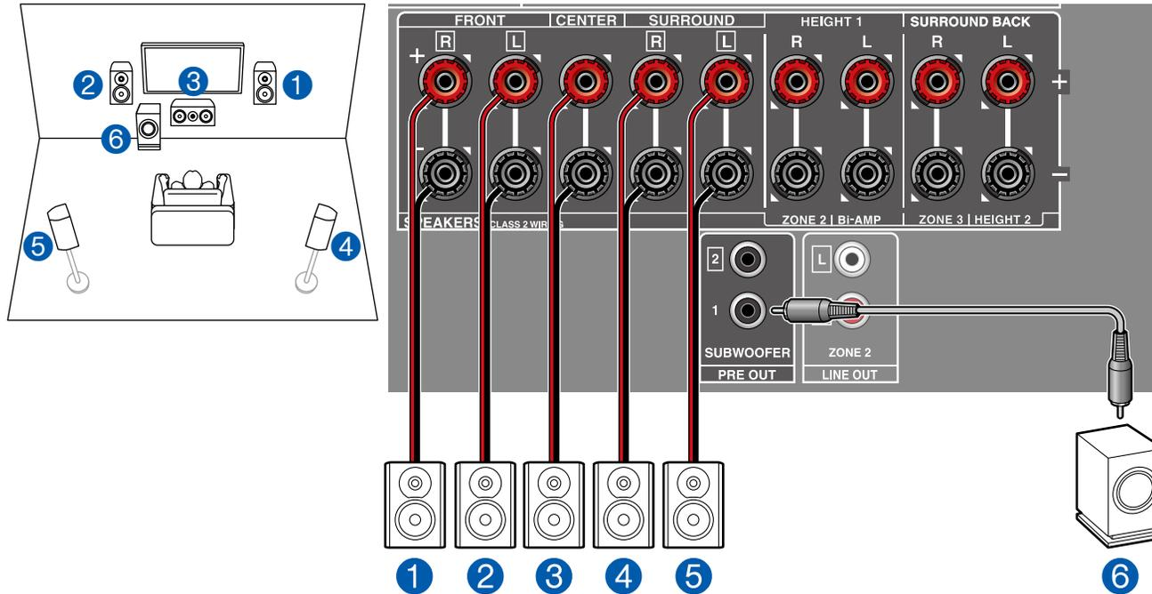
This is a basic 5.1 Channel System. For details of the speaker layout, refer to "Speaker Installation" (→p14).
