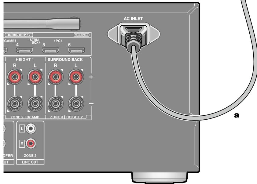
Connect the power cord after all the connections are completed.
