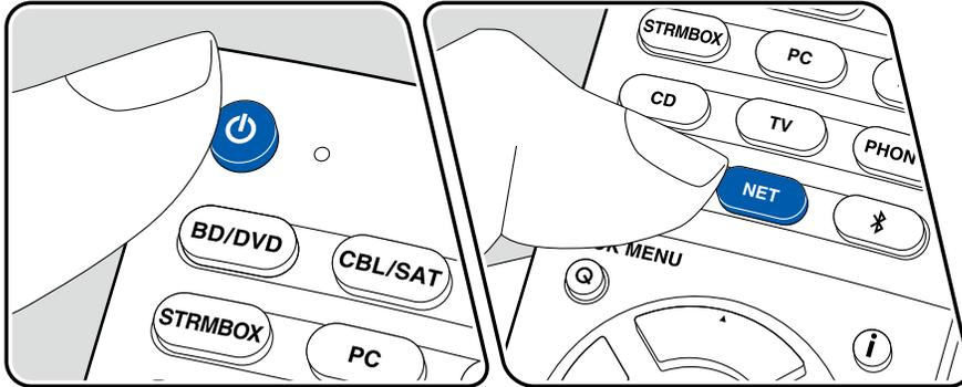
Set the remote controller to the ZONE control mode (ZONE 2/ZONE 3) (→p82, 83), and then perform the following operations.
