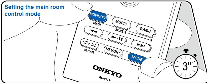
At the time of purchase, the remote controller is in the mode to control playback in the main room. To play a source in ZONE 2, set the remote controller to the ZONE control mode (ZONE 2). To control the main room play again, restore the remote controller to the main room control mode.
