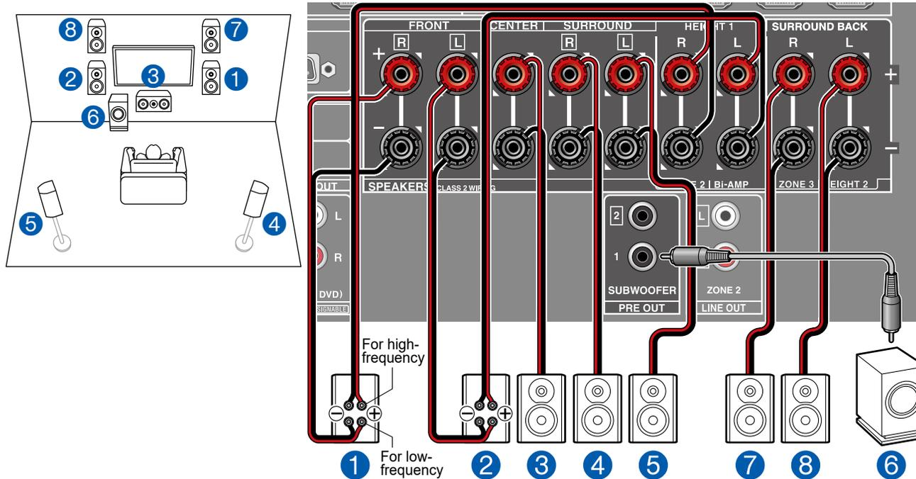
This is a combination of the 5.1 Channel System and front high speakers. A front high speaker is a type of height speaker. You can select only one set of height speakers from the following three types for connection.
