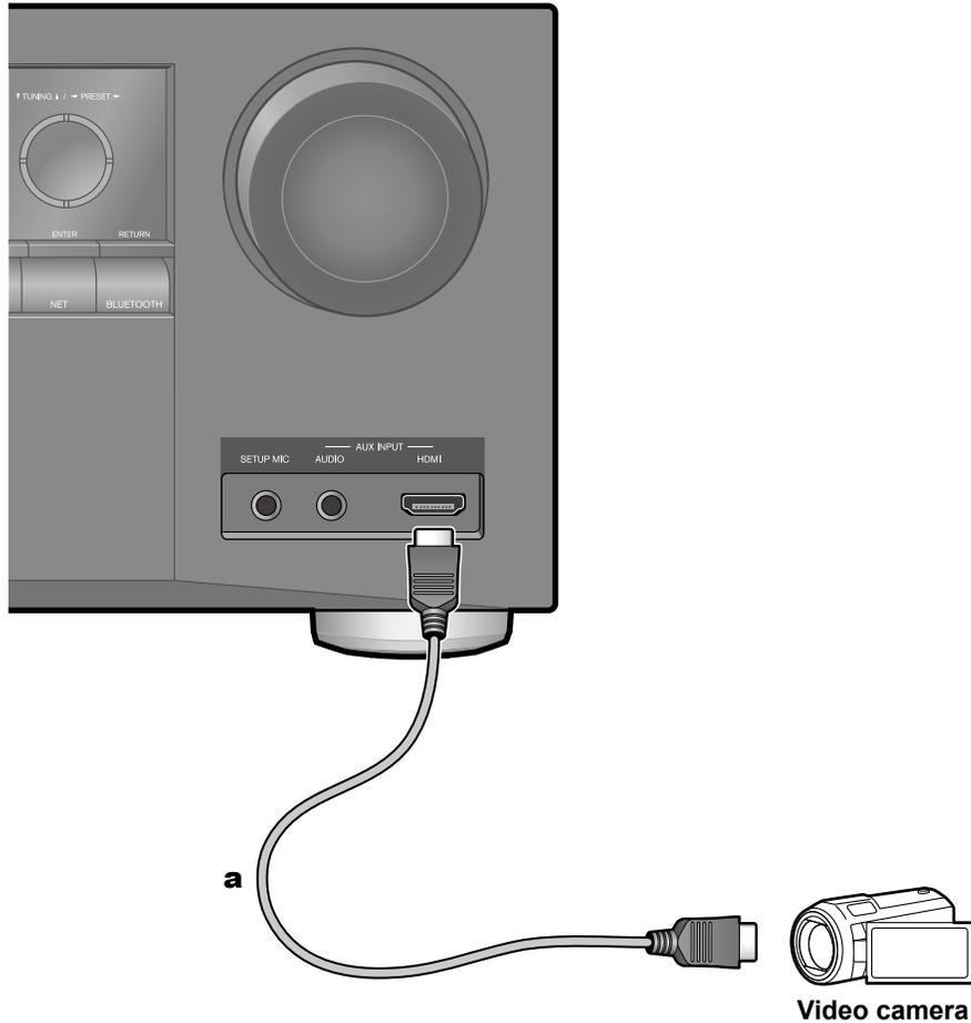
Connect a video camera, etc. to the AUX INPUT AUDIO/HDMI jack on the front panel using an HDMI cable or stereo mini plug cable ( $\varnothing 1/8''/3.5$  mm).
