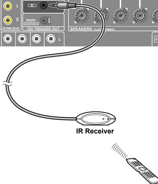
When connecting a remote control receiver unit consisting of an IR Receiver, etc. to this unit, operation using the remote controller is possible even if the remote control signal is difficult to reach (due to installation in the cabinet, etc.). You can also operate the unit using the remote controller from a separate room such as ZONE 2. For adopting a remote control receiver unit, contact the specialized stores.
