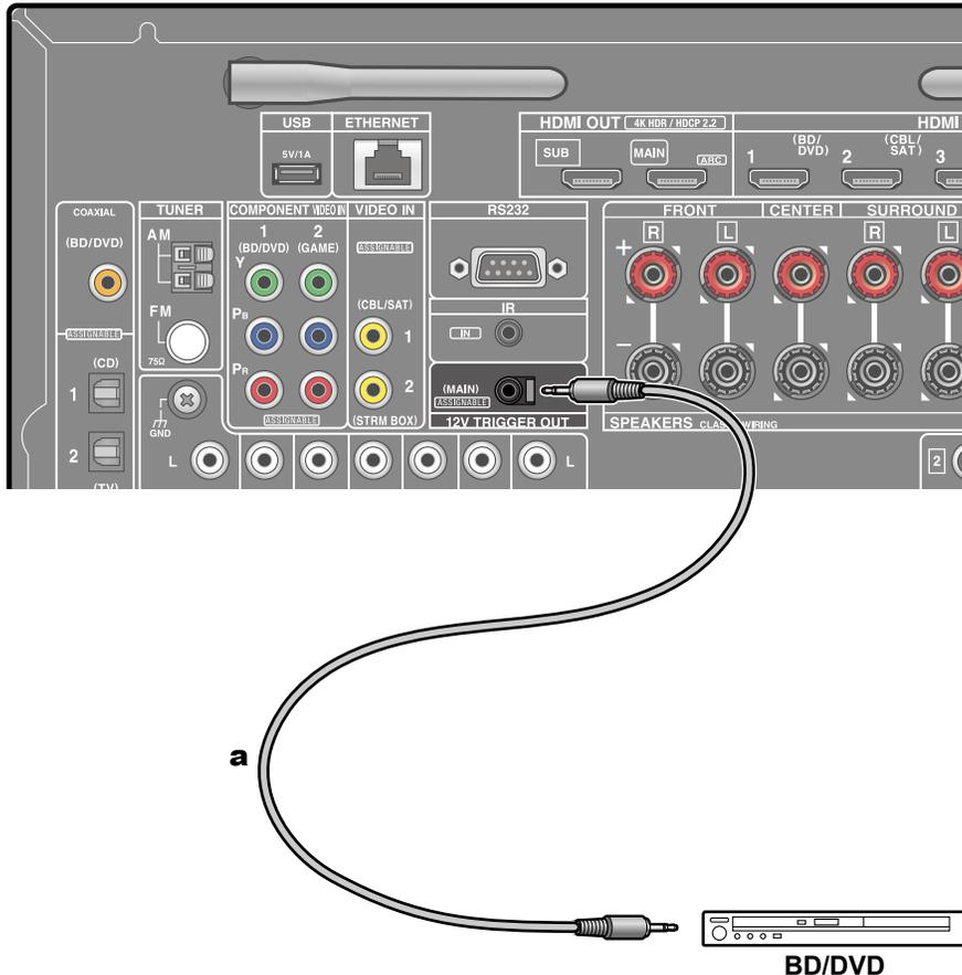
When connecting a device equipped with a TRIGGER IN jack such as a BD/DVD player to this unit, the device can be turned on or set to standby by interlocking the operation on this unit. When any input is selected, this unit outputs a maximum of 12 V/100 mA control signal from the 12V TRIGGER OUT jack, and controls the power link operation of the external device.
