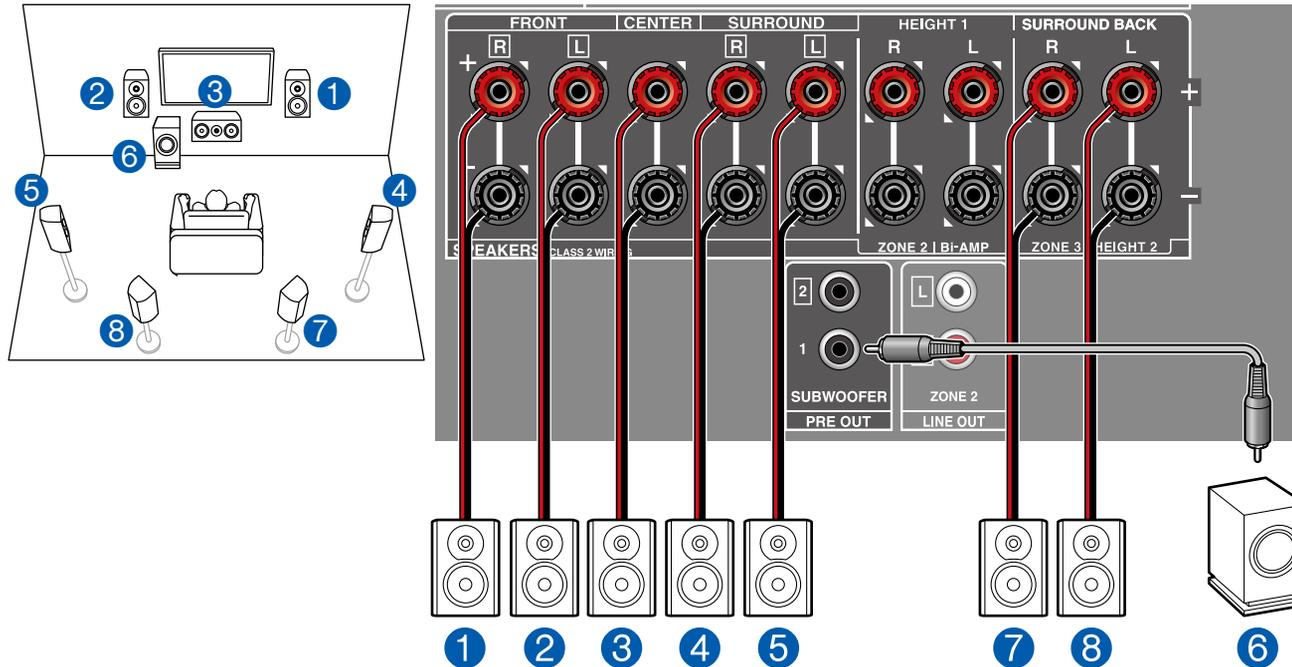
This is a 7.1 Channel System that consists of the basic 5.1 Channel System and added surround back speakers. For details of the speaker layout, refer to "Speaker Installation" (→p15).
