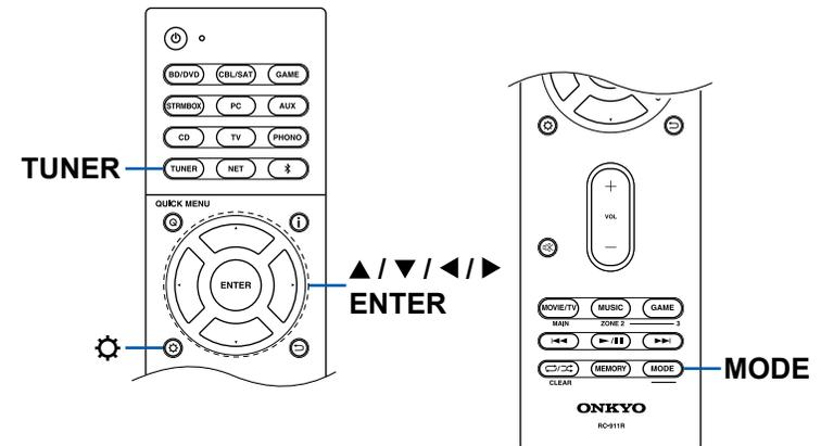
**When FM broadcasts reception is poor:** Perform the procedure for "Tuning Manually" (→p79). Note that if you tune manually, the reception for FM broadcasts will be monaural rather than stereo, irrespective of the sensitivity of the reception.
