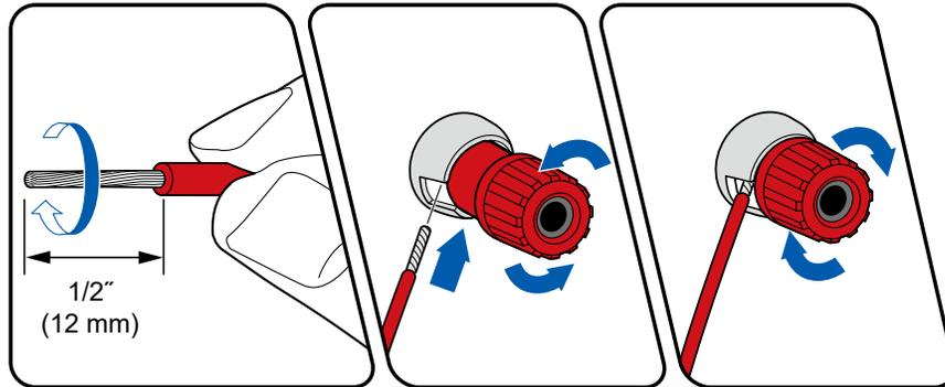
Make correct connection between the unit's jacks and speaker's jacks (+ side to + side, and - side to - side) for each channel. If the connection is wrong, a bass sound will not be reproduced properly due to reverse phase. Twist the wires exposed from the tip of the speaker cable so that the wires do not stick out of the speaker terminal when connecting. If the exposed wires touch the rear panel, or the + side and - side wires touch each other, the protection circuit will be activated.
