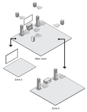
● The sources from which you can enjoy the sound in a separate room: For Zone 2, any can be selected from among an external device connected to the HDMI input jack or the analog audio input jacks (\*) of the unit, the "NET", "USB" or "BLUETOOTH" source, and the AM/FM broadcasting. For Zone 3, any can be selected from among an external device connected to
