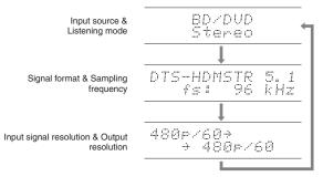
If "Dolby D 5.1" is displayed in signal format, the Dolby Digital 5.1 ch signals are being input. When listening to AM/FM radio, the band, frequency and preset number are displayed.
