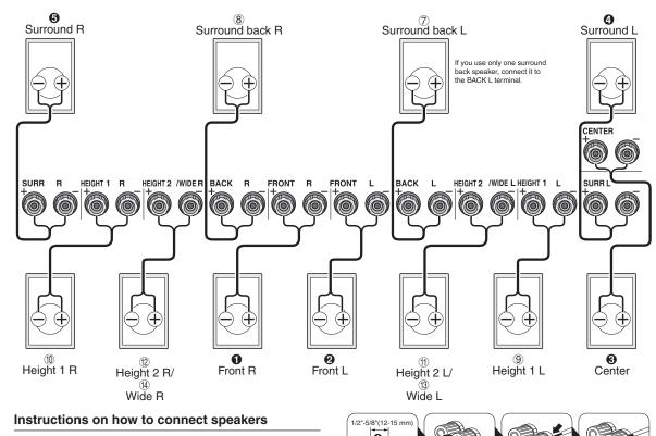
Important: Connect speakers with 4  $\Omega$  to 16  $\Omega$  impedance. You have to change the setting if any of the speakers have 4  $\Omega$  or more to less than 6  $\Omega$  impedance. You can set up by viewing the guidance displayed on the TV screen. Press RECEIVER and then HOME on the remote controller. Select "Setup" - "2.Speaker Setup" - "Speaker Settings" - "Speaker Impedance" and change the default value from "60hms" to "40hms".
