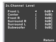
Adjust the level of each speaker as the test tone is emitted.
