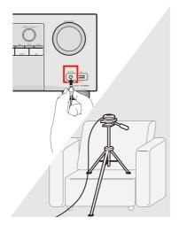
If you have a tripod, use it to place the microphone so that it's about ear level at your normal listening position. Otherwise, place the microphone at ear level using a table or a chair.
