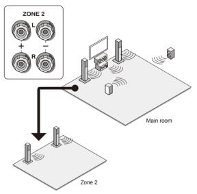
These settings are required: After connecting the speakers, press (RECEIVER and then SETUP on the remote controller, select "2. Speaker" - "Configuration" and set "Powered Zone2" to "Yes".
