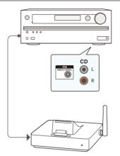
Connect an Onkyo component with RI jack to this unit using an RI cable and an analog audio cable. For details, refer to the instruction manual of the component with RI jack. The RI cable can be connected in any order. When there are two RI jacks, both jacks work in the same way and are interchangeable.
