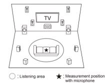
\* Correct measurement will not be possible if the microphone is held by hand. Measurement is not possible if headphones are being used.
